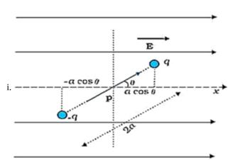
The amount of work done in rotating the dipole from  $\theta = \theta_0$  to  $\theta = \theta_1$  by the external torque
